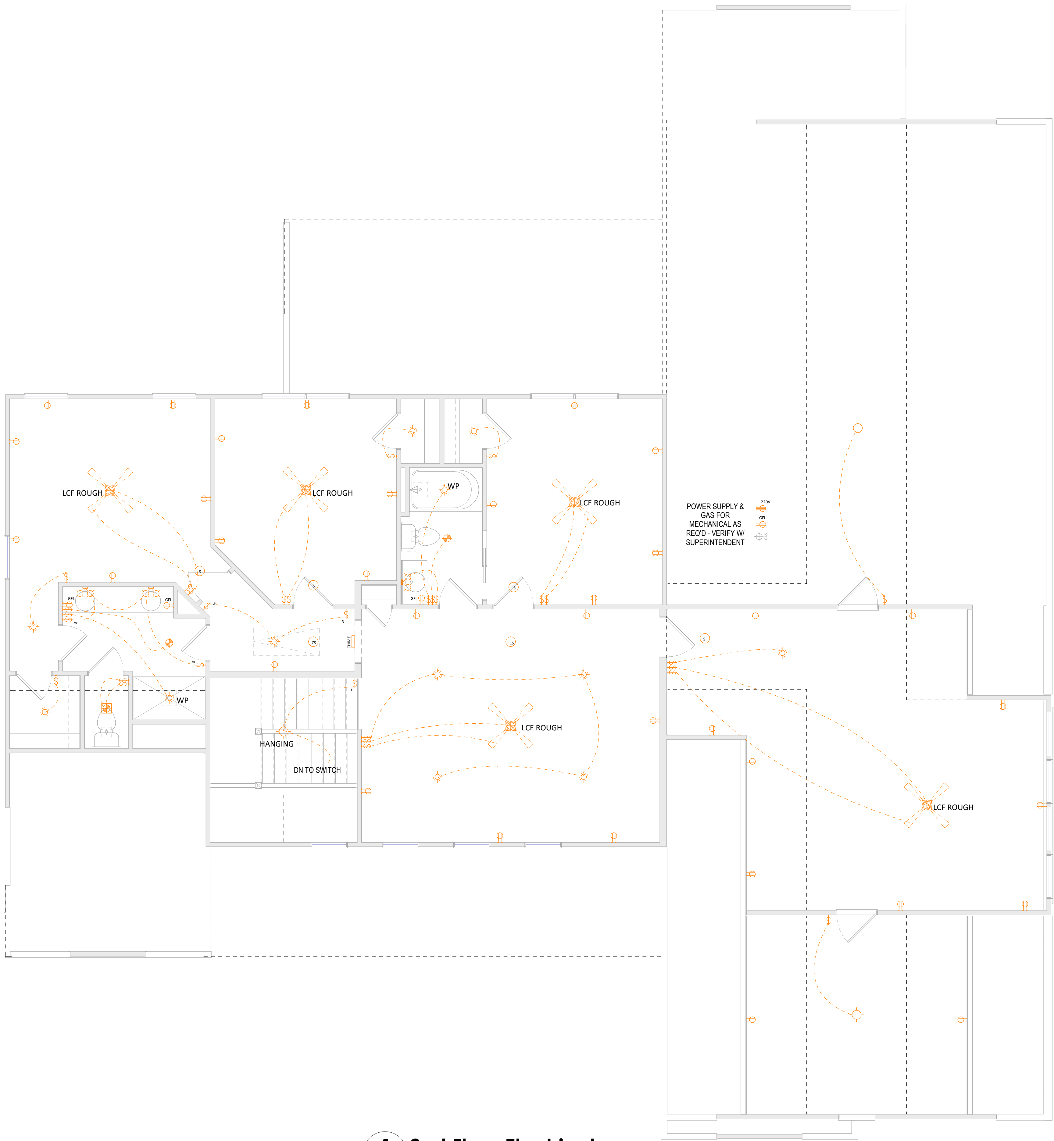
1 2nd Floor Electrical A-5.2 1/4" = 1'-0"
